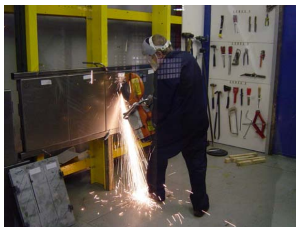
Secure Walling panel delay factor tests. Simulated attack by heavy duty angle grinder.
