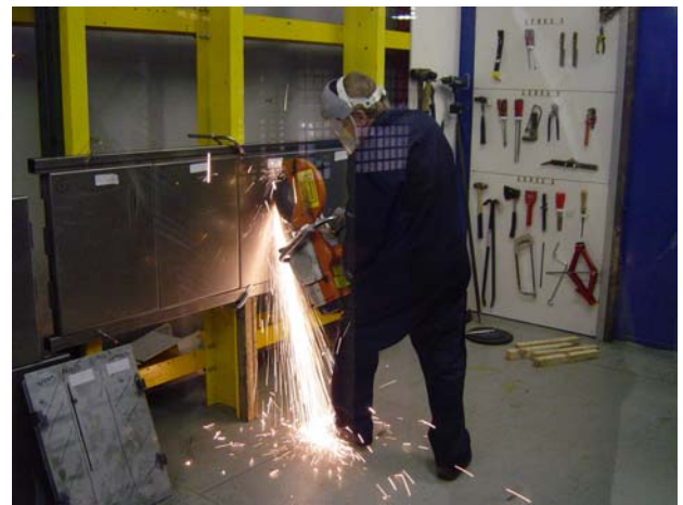
Secure Walling panel delay factor tests. Simulated attack by heavy duty angle grinder.
